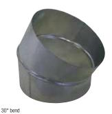
**Product description** The 30° bend is used to change the direction of a galvanised ducting system by a 30° angle. Up to diameter 200 mm, bends are pressed; diameter 250 to 900 are sector bends.
