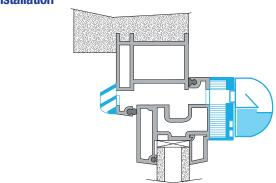
Cross-section of spacer installation
