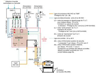
Schematic drawing of a system featuring a 2-speed smoke and heat exhaust box fan with progressive start
