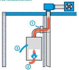
1. Burner off: the default ventilation airflow no longer passes via the boiler, a specific port on the  $\ensuremath{\mathsf{BAZ}}$  Pilot is used, 2. Burner lit: the terminal draws a sufficient airflow through the boiler to remove the burnt gases, 3. Whatever the state of the burner: a push button can be used to activate a peak ventilation airflow drawn over the boiler.
