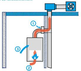
1. Burner off: the default ventilation airflow no longer passes via the boiler, a specific port on the  $\ensuremath{\mathsf{BAZ}}$  Pilot is used, 2. Burner lit: the terminal draws a sufficient airflow through the boiler to remove the burnt gases, 3. Whatever the state of the burner: a push button can be used to activate a peak ventilation airflow drawn over the boiler.
