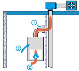
1. Burner off: the default ventilation airflow no longer passes via the boiler, a specific port on the BAZ Pilot is used, 2. Burner lit: the terminal draws a sufficient airflow through the boiler to remove the burnt gases, 3. Whatever the state of the burner: a push button can be used to activate a peak ventilation airflow drawn over the boiler.
