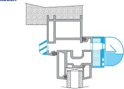
Cross-section of spacer installation
