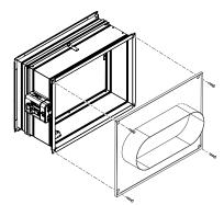
Installation of oblong ring on mechanism side of the ISONE 2 damper
