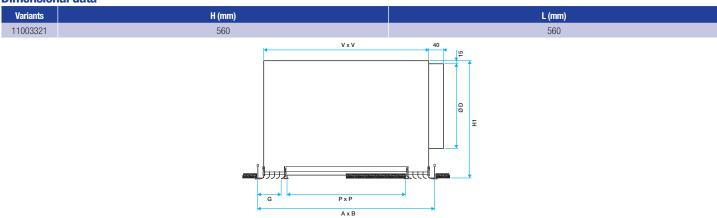
Dimensions of RE 610 plenum with diffuser
