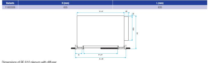
Dimensions of RE 610 plenum with diffuser
