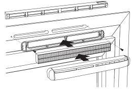
Installation of AirFilter®
