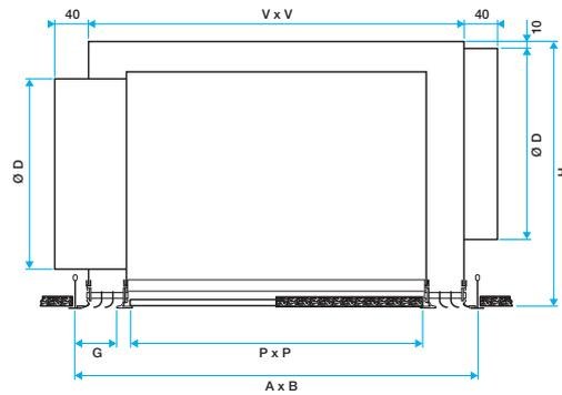
Dimensions of R-RE plenum with ALD diffuser fitted
