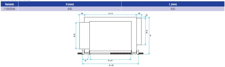
Dimensions of R-RE plenum with ALD diffuser fitted
