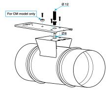
Installation of motor plate
