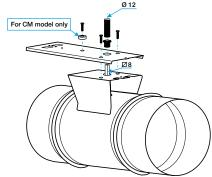
Installation of motor plate
