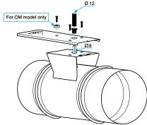
Installation of motor plate
