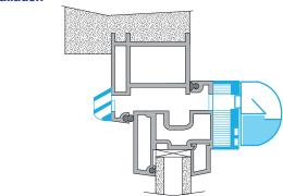
Cross-section of spacer installation
