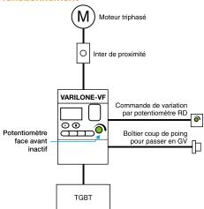
Varilone is controlled by a potentiometer to vary the speed and a «punch» button to switch to maximum airflow for smoke and heat exhaust.
