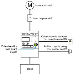
Varilone is controlled by a potentiometer to vary the speed and a «punch» button to switch to maximum airflow for smoke and heat exhaust.
